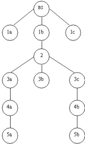
Figure 14: Five level deep reference multihop network with 11 nodes. Edges represent bidirectional connectivity.
