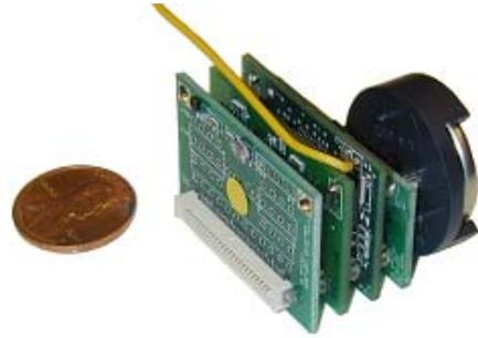
**Figure 1: Our low-power networked sensor device prototype.**
