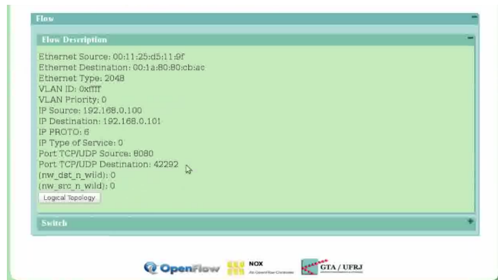
Figure 6.12: Flow description after a flow search. The Logical Topology button provides a graphical visualization of the flow.
