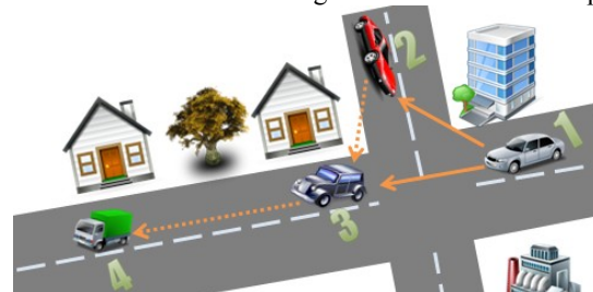
Fig. 3. The two nodes 2 and 3 retransmit the packet received from node 1. Even node 2 is the farthest compared to node 3, DHVN rebroadcasts the message in each direction, so node 4 will also receive it from node 3.
