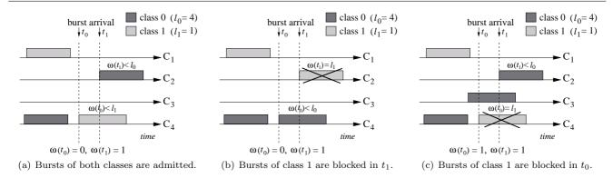
Fig. 2 Examples of how the load-level-based mechanism works.
