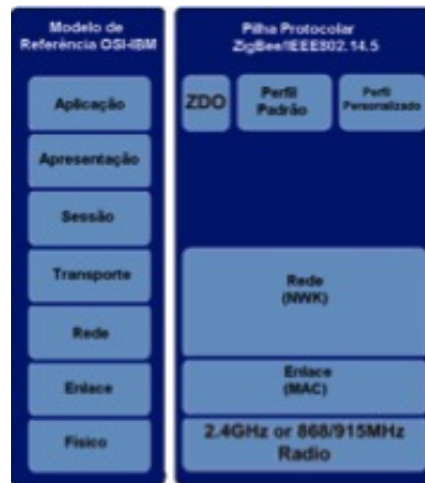
Figura II.3: Camadas OSI X Zigbee. [1]
