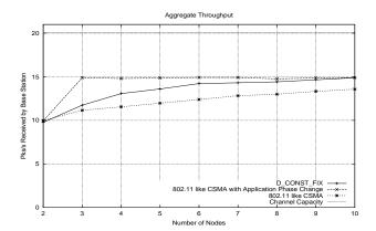
Figure 9: Aggregate throughput comparison between 802.11 CSMA and 802.11 CSMA with application phase change.
