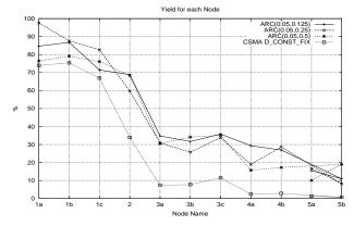
Figure 22: Percent yield (packet received by base station/packet transmitted) of each node. (Empirical)
