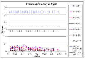
Figure 16: Variance, a measure of fairness, of the bandwidth received by the base station from each node.
