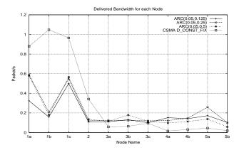
Figure 20: Delivered bandwidth received by the base station from each node. (Empirical)
