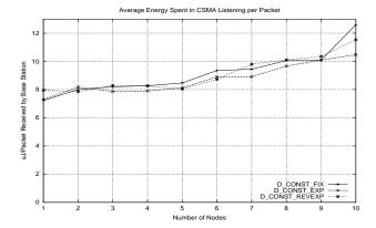
Figure 12: Actual energy spent in CSMA listening over our network sensor prototypes for the different CSMA schemes.(Empirical)
