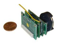
Figure 1: Our low-power networked sensor device prototype.
