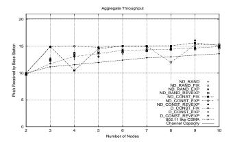
Figure 4: Aggregate delivered bandwidth for CSMA schemes with typical start conditions and offered load of 5 packets per second per node.
