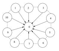
Figure 3: Network topology for the evaluating the CSMA scheme.
