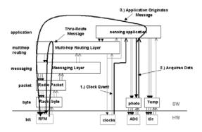
Figure 2: Complete TinyOS application component graph.
