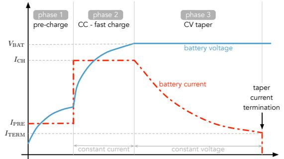
Fig. 1: Li-ion battery charging profile.
