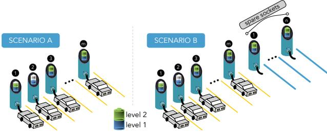
Fig. 2: Charging stations scenarios, traditional (A) and with spare capacity reuse (B).
