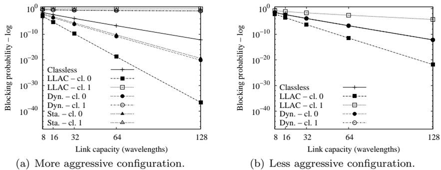
Fig. 11 Impact of the link capacity.
