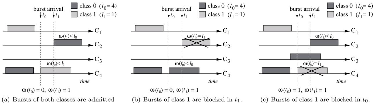
**Fig. 2** Examples of how the load-level-based mechanism works.
