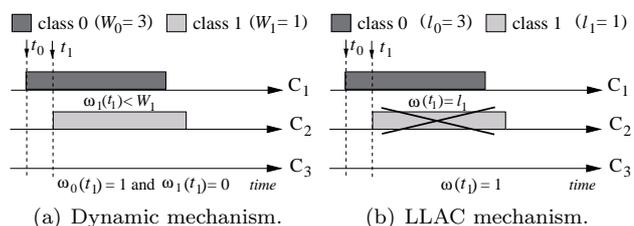
**Fig. 3** Load-level-based mechanism vs. dynamic mechanism.
